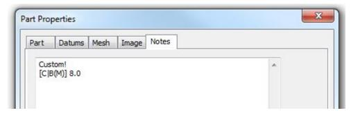
If the gage diameter is not explicitly specified as **8.0**, then the datum reference frame gage diameter of **7.89** (the virtual condition of 8.0 - 0.01 - 0.1) is used.
