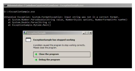
As you can see, the System.Number.ParseDouble function raises a System.FormatException, complaining that the input string was not in a correct format. The exception is not handled, so it is passed up the call stack to the System.Double.Parse function, which again does not handle it. Eventually, the exception reaches our MyCode.Main function, where it again goes unhandled, so our program crashes.
