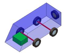
As you can see, the car consists of an engine (the green block), an exterior shape (the blue thing), two axles, and a spare wheel. Each axle consists of a shaft and two wheels. The exterior shape is a sheet body in Car\_Assembly.prt, so you don't see it in the Assembly Navigator. Similarly, the red shaft is a solid body in Axle\_Assembly.prt, so you don't see this, either.
