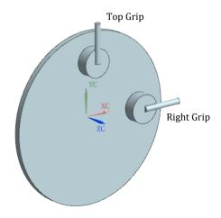
We create a new assembly part and insert the door component into it, just as before. Next, we have to position and orient the two handles as shown below:
