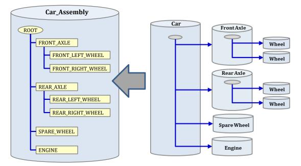
The yellow items are called "**Components**" or sometimes "**Part Occurrences**". The tree of components inside a part file replicates the tree structure of the subassemblies themselves. So, if we want to know about this structure, we can simply traverse through the tree of component objects in the file, without opening any other part files.
