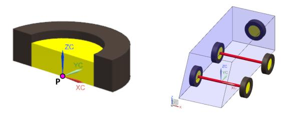
When the front left wheel gets inserted into the car assembly, this point P gets placed at (950, 0, 0). So, if comp is the FRONT\_LEFT\_WHEEL component, then comp.Position is (950, 0, 0). Similarly, the REAR\_LEFT\_WHEEL component has Position = (950, 2000, 0).
