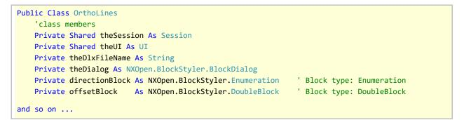
As you can see, we are defining a new class called "OrthoLines" to represent instances of our dialog. Notice that there are two lines that declare variables called directionBlock and offsetBlock to hold the two blocks that make up an "OrthoLines" dialog.
