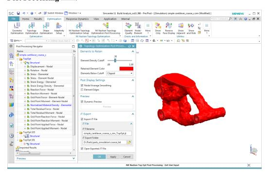
4. To add or remove elements based on their element density, move the **Element Density Cutoff** slider to the left or right.
